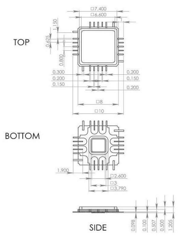
Fig. 2. CQFP 24-Pin Package Drawing (All Dimensions in mm)
