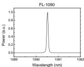
The FL-1090 is an Ytterbium fiber laser that delivers up to 6 W optical power at 1090.5 nm wavelength. The laser cavity is made by fiber Bragg reflectors that don't require any alignment and the system includes the pump source and the control electronics.
