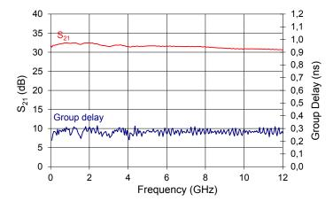
$S_{12}$  Parameter Curve Conditions:  $V_{bias} = 12 \text{ V}, V_{amp} = 1.2 \text{ V}, I_{bias} = 310 \text{ mA}$
