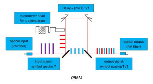
We add a variable optical attenuation (VOA) in order to equilibrate the insertion losses in each path. A variable optical delay (VODL) can also be added:
