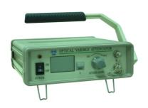
Accelink's Benchtop Variable Optical Attenuator support continuously attenuation of optical signals at the calibration wavelengths of 1310/1550nm, and the attenuation setting is indicated on a large LCD, the attenuation level is hold when the power is turned on or off. It is a compact, portable instruments for field applications as well as in laboratory applications.
