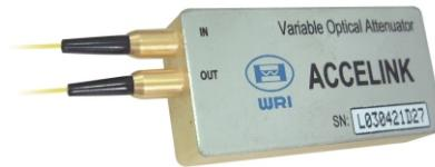
Accelink's Volatage Controlled Optical Attenuator(EVOA) is designed to optimize the optical signal power of at key points of optical communication networks. It is a new miniature variable attenuator for either Cor L band applications. The attenuator offers high thermal stability, compact size and excellent reliability. The products meet the Telcordia GR-1221-CORE requirements.
