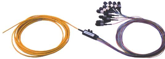
Optical Fiber Ribbon Fan-out Pigtail can separate and protect fibers in a multi-core optical fiber ribbon (such as 12 cores) through a special fan-out splitter, so as to connect each fiber through a connector to make the fibers connection on ODF.
