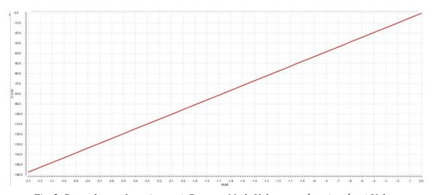
Fig. 2. Dependence of cep (or cen) Common Mode Voltage on dccp (or dccn) Voltage
