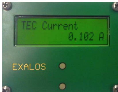
Fig. 10 Display-Board DIB5000 in display mode 4 (TEC current)
