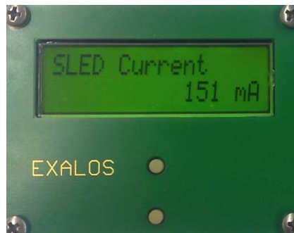
Fig. 7 Display-Board DIB5000 in default display mode 1 (SLED drive current)
