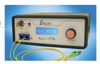
The XLT-BFA Series of amplifiers is the high-power solution offered by EXELITE Innovations. The XLT-BFA Fiber Amplifiers are easy-to-use and are specially designed to offer high optical power and low noise signal levels for optical transmission and non-linear applications in the C-band.
