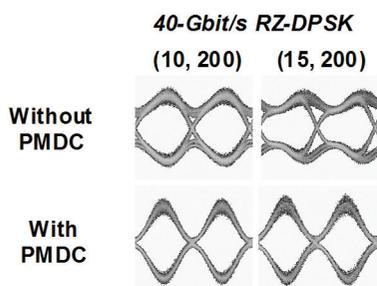
Figure 3. Captured eye diagrams of 40-Gbit/s RZ-DPSK signals with and without PMDC. (15, 200) represents 15 ps DGD and 200 ps<sup>2</sup> SOPMD.
