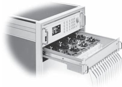
*When coupled with the LDM-4616 Modular Laser Diode Mount, the LDC-3916 Multi-channel controller provides a configurable, cost-effective solution for multi-channel, DWDM signal sources. This mount can also support many popular 980nm and 1480nm pump laser diodes for EDFA test applications.*
